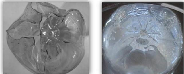
Figure 1. Typical failure region on carbonated soft drink containers.
