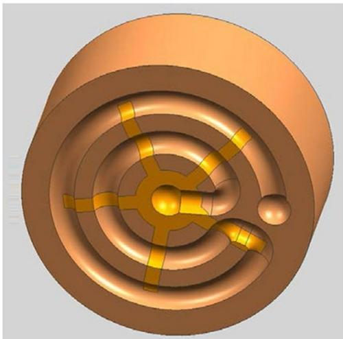
**Figure 7.** Base cooling option with copper insert
