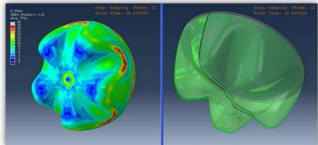
Figure 2. Modeled stress and deformation in a petaloid base under internal pressure
