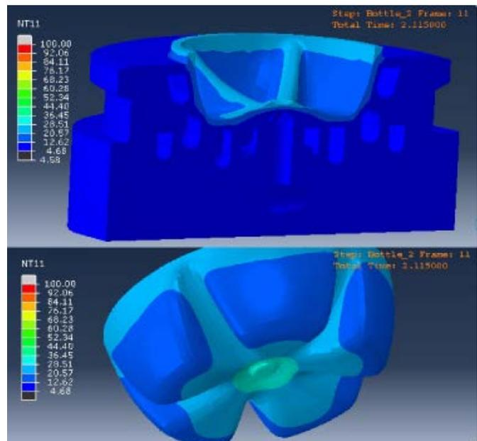
**Figure 6.** Simulated Temperature distribution in the plastic part and the metal mold during a quenching cycle
