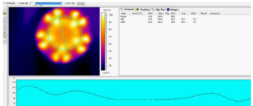
**Figure 9.** Petaloid bottle base temperature monitored with a Thermal Imaging camera
