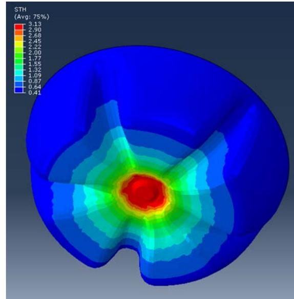
**Figure 5.** Predicted Petaloid base thickness distribution plot
